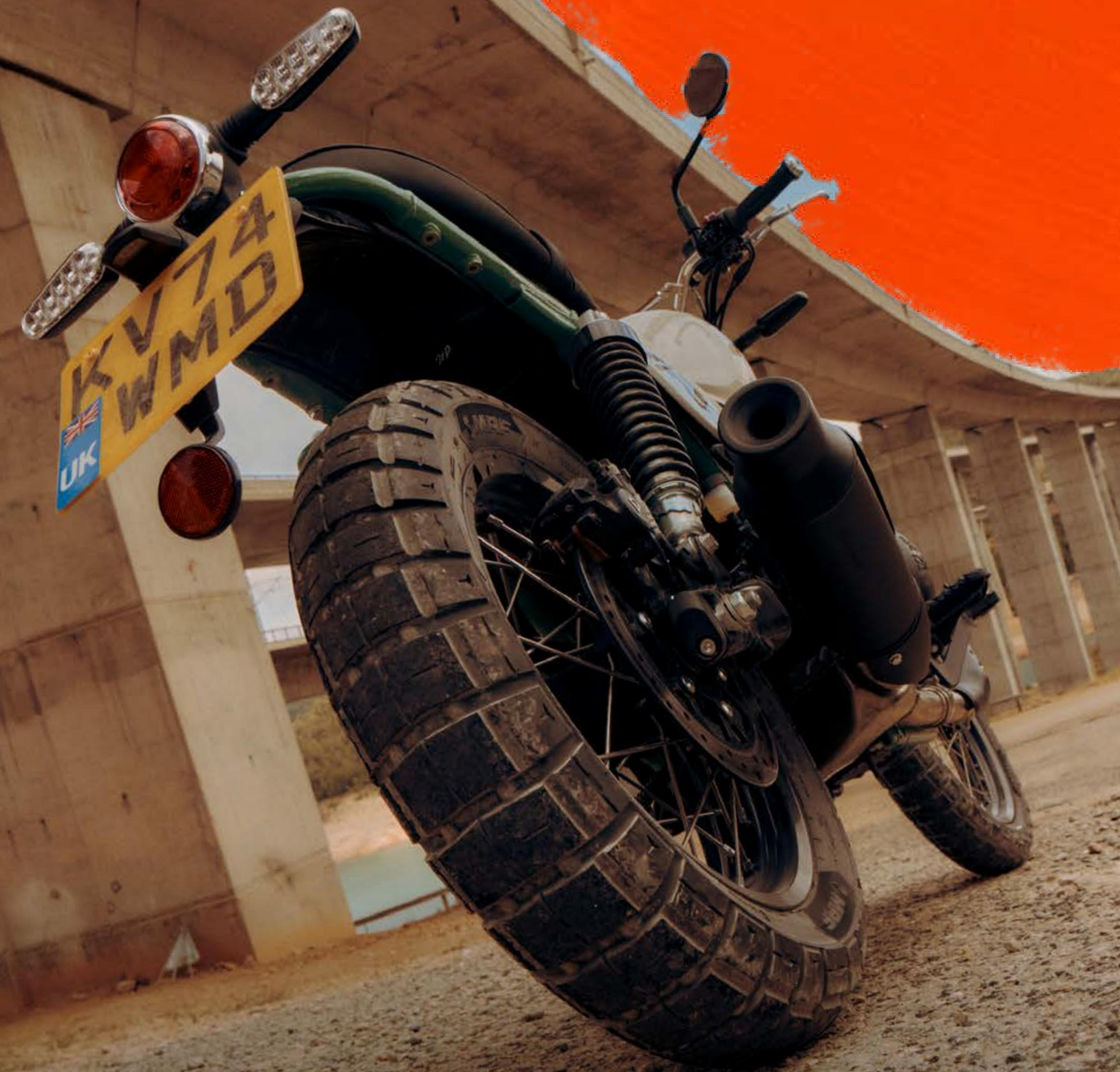
Chunky dual purpose tyres are a key scrambler feature. They provide more grip on loose surfaces without losing confidence on tarmac. The open square tread blocks give a retro flavour.
